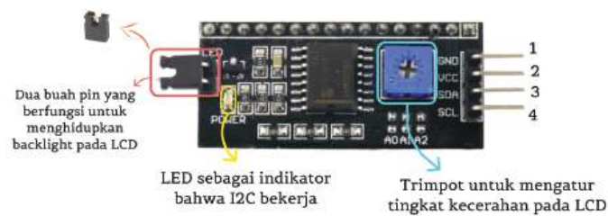
Gambar 9.21 Pin Modul I2C
